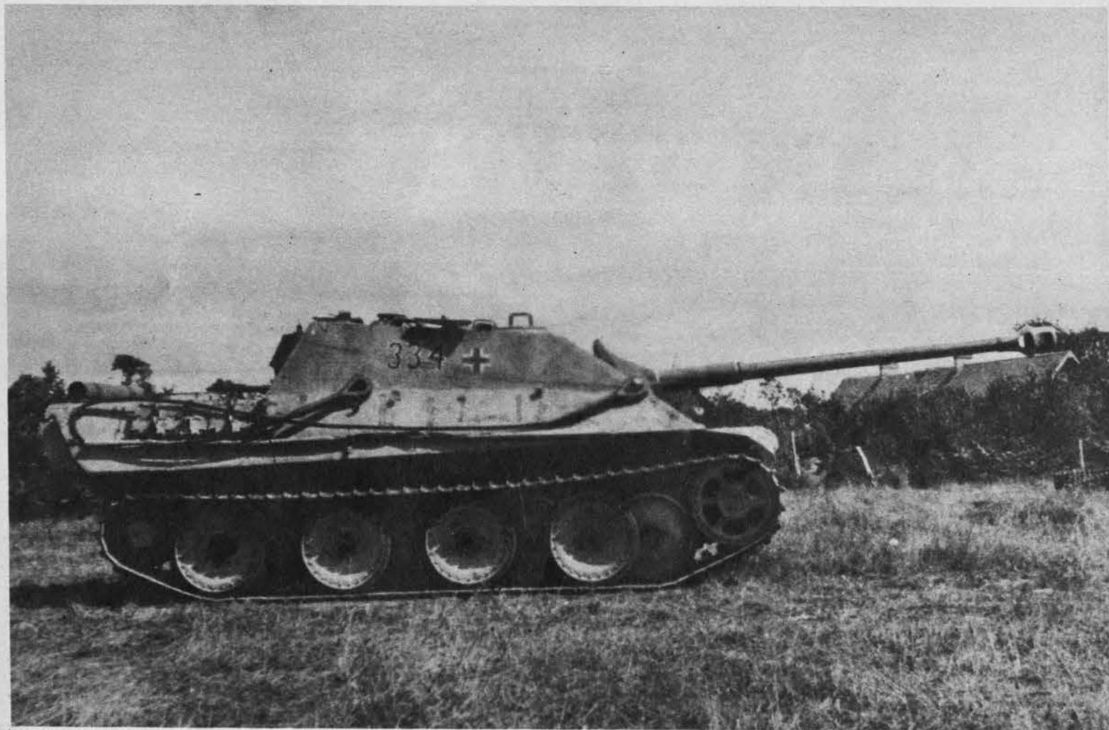
Low silhouette makes Hunting Panther hard to hit, easy to dig in for antitank defense. The chassis is same as that of the Panther tank, but
